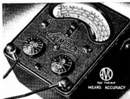
The 50-range Model 7 Universal AvoMeter.
